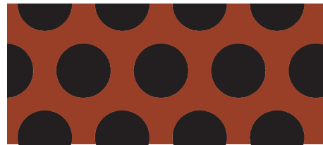
A25 3/8" holes | 9/16" staggered centers 40% open area | Shown in Mission Red
