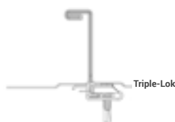
FLS Series standing seam panel features a Triple-Lok design
