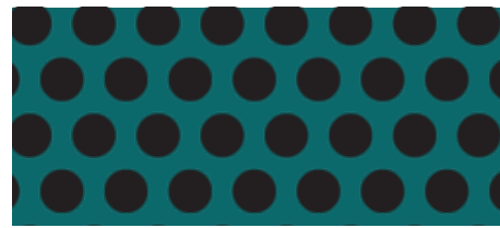
A19 3/16" holes | 5/16" staggered centers 33% open area | Shown in Teal
