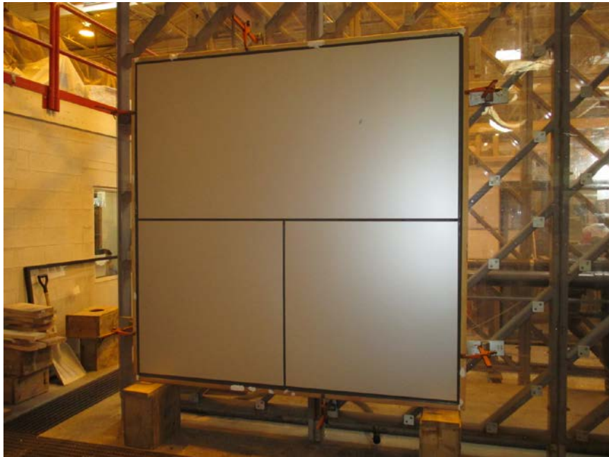
Photo No. 1 View of Tested Wall Assembly
