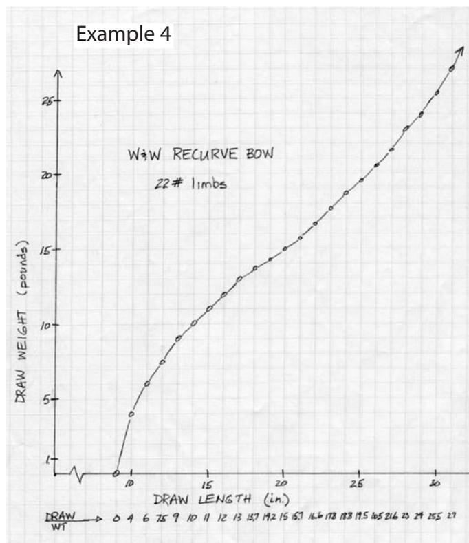
This Win & Win recurve does not have a straight-line draw curve like the long bow would. As the recurve limbs unbend they allow for a less steep weight increase mid-way through the draw stroke. As you draw the recurve further the increase gets steeper which is called “stacking”. Note that I used a one pound vertical scale for this light-weight recurve.
