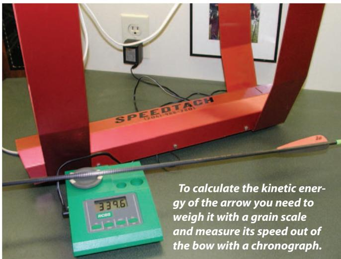
To calculate the kinetic energy of the arrow you need to weigh it with a grain scale and measure its speed out of the bow with a chronograph.
