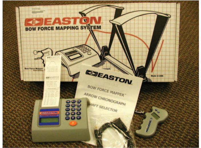
*Easton has a complete kit to make stored energy calculation easy. The Mapper Kit contains a hand held digital scale unit, a chronograph and a printer unit. Draw the bow with the digital scale and it records the draw weight data that you can download into the printer. This great kit provides the chronograph to measure arrow speed data but you'll have to have your own grain scale to weigh the arrow.*
