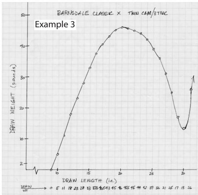
A Barnsdale twin-cam bow increases to peak weight over a longer distance and drops smoothly into the “valley” or holding weight. Notice the recorded draw weight data along the bottom line of the graph page.
