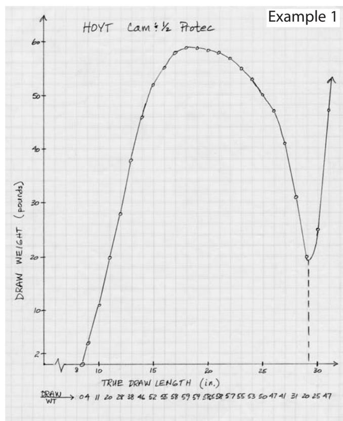
This force-draw curve was made for my Hoyt Cam & 1/2 Protec. As you can easily see, the draw weight increases rapidly at the beginning of the draw stroke and stays near peak weight for five or more inches before letting off to the holding weight at 29.25 inches of true draw length (31" AMO draw length). Beyond this point, the weight increases dramatically as the cables hit the cam draw-stops. Notice that the draw weight is scaled vertically in two-pound increments.
