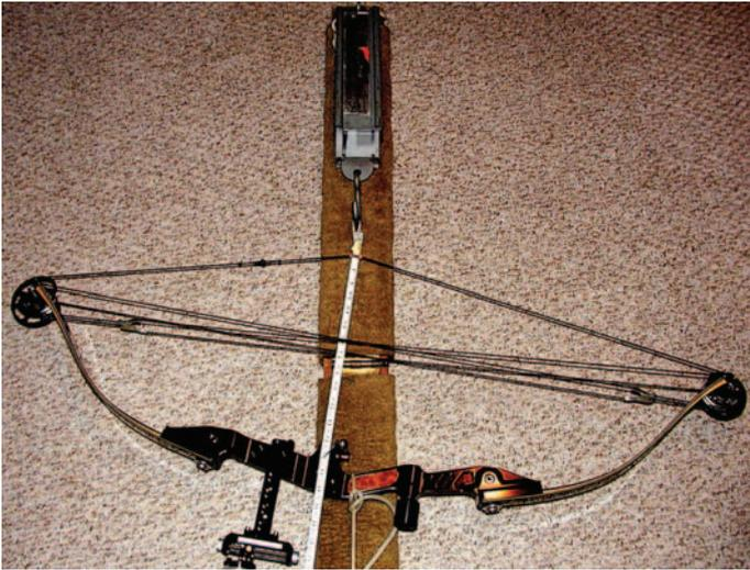
*To collect the data for a force-draw curve you could build the device shown here. A spring-scale is attached to the top of a six-foot 2x4 and a winch at the other end. The bow is hooked to the scale by the bowstring and a rope is used to hook the riser to the winch. As the winch is turned a tape measure indicates how far the bow is being drawn. Recording the weights at each inch of draw length is all you need to build a graph.*
