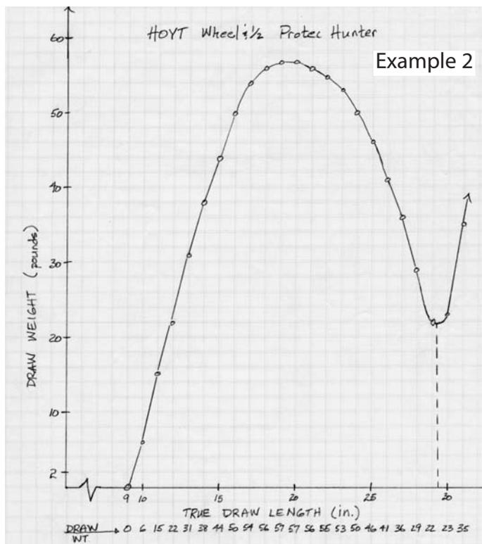
I hunt with this Hoyt Wheel & 1/2 Protec because it's easy to draw when I'm cold but yet provides plenty of energy for the arrow. Notice the rounded-top to the curve indicating that this bow stores a little less energy than a cam bow but is easier to draw over peak weight for us old guys with worn-out shoulders. It also has a softer feeling, rounded valley which I like but most don't.
