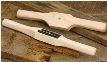
*The Smooth Scraper was designed specifically for bowbuilding. The handle and sharp blade combination is the secret to success for this handy little tool. The Mystic Scraper at right is unlike regular cabinet scrapers in that it's thick and inflexible, yet turns a nice fine shaving.*
