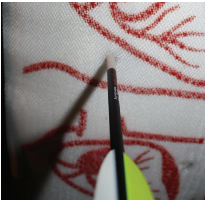
A photograph of typical penetration into the target after 28 shots from close range into the same hole.
