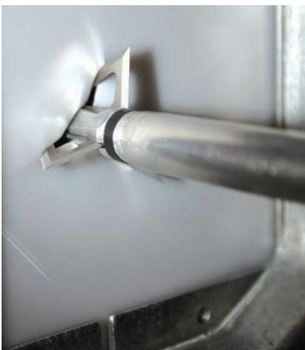
The force needed is recorded from tip to shaft as the broadhead penetrates the multiple layers of poly sheeting.
