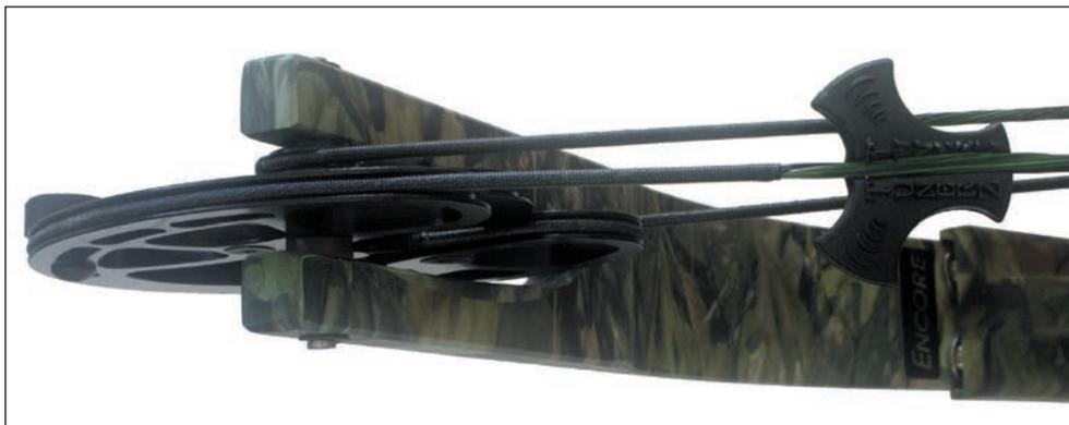
**Chuck Nease designed the TAC Cam System so a minimum of components are needed (below) to make the switch between twin cam and hybrid systems. If you order the Encore II as as Twin Cam model, you can press the bow and remove a module from the lower cam, then replace one cable with a take-up string. You'll make some adjustments on cable and take-up strings to get things set up but in most cases, you won't need to adjust the nocking point.**
