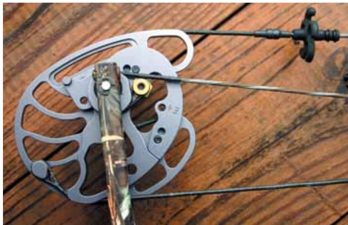
*The Tribute, like all BowTech models for 2006, uses the Binary Cam system invented by VP and Co-Founder Kevin Strother. Instead of splitting the buss cable with a yoke to anchor on the axle ends, the buss cable ends in the opposite cam.*
