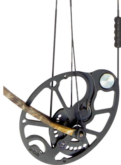
*Designer Matt McPherson used stainless steel perimeter weights in both cams, to help give the Menace the shock-free feel of a parallel limb bow, without the cost and weight of the long riser that would be used with parallel limbs. Note the speed buttons, how the adjustment holes are in a single line and how the cable falls across the timing hole in the outer portion of the cam. The single cap head screw needs no lock washer since the metal has been dished out to provide self-locking.*
