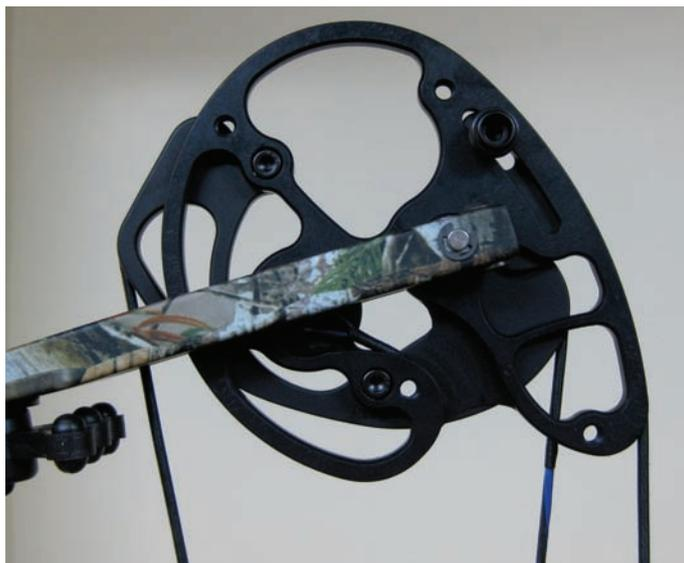
**Quest outfits the Primal with their SYNC Two-Track Cam system. The cables share a track on each cam and are forced to work together as they are both anchored on both ends to the eccentrics. The result is a self adjusting cam system that requires little maintenance.**
