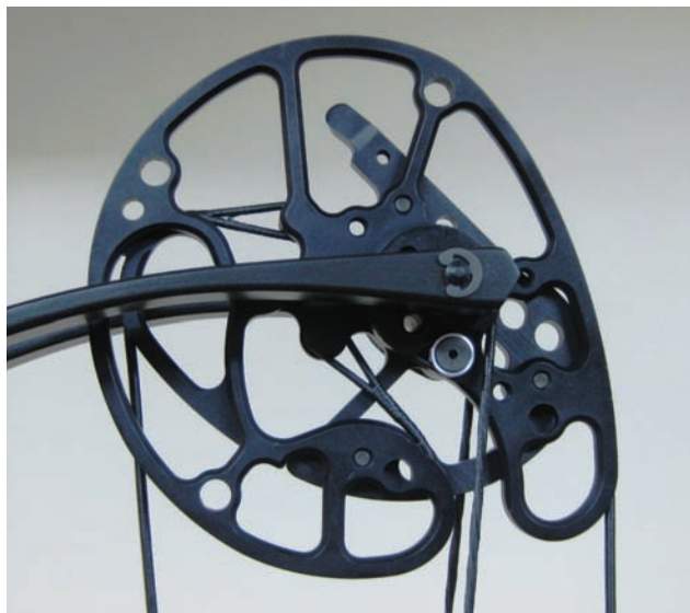
The DS 3800 is driven by Darton’s DualSync High Efficiency Synchronized Dual Cam System. Working with other technologies on the bow this cam system cranks out advertised IBO speeds between 345 and 350 fps. Draw lengths are easily adjusted through a set of modules that do not require a bow press to change out. This view also shows the cable straddling the cam to equal out the tension and reduce limb twisting torque.
