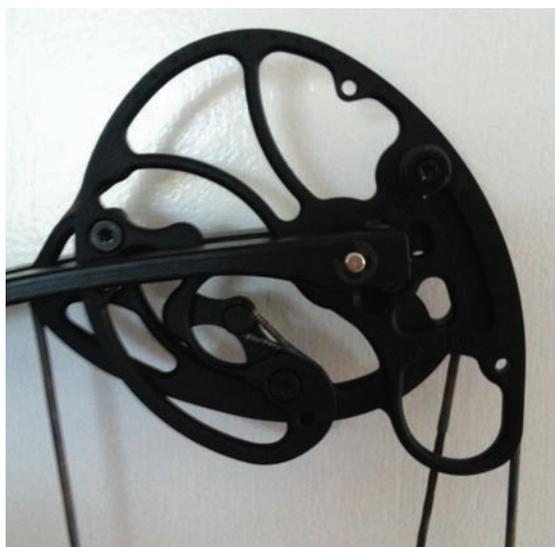
**Strother's Hyper-S cam is designed to keep the applied load near the center of the axle thereby reducing the opportunity for efficiency robbing limb twist and cam lean. On the SX-1 the two cams are harnessed together in a Dual Sync system.**
