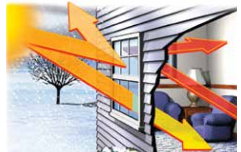
Winter Energy Savings: Low-E insulating glass reduces heat loss by reflecting warm air back into your home.
