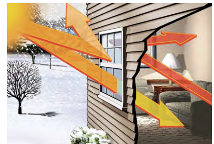
During the winter, Low-E insulating glass reduces heat loss by reflecting warmth back into your home.
