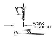
2. **Work Through** – is the distance from the pin line to the front of the seat at the front stops.
