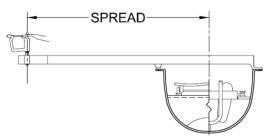
1b. **Spread** (sweep) – is the distance from the centerline of the boat to the centre of the oarlock pin measured perpendicular to the boat.
