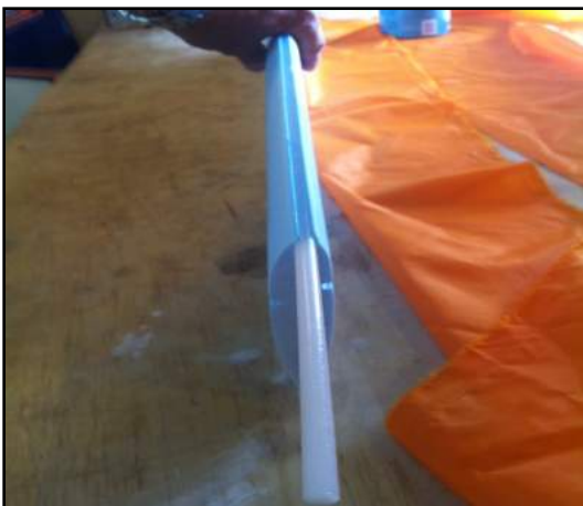
Figure 8 Insert Leading Edge plastic rod
