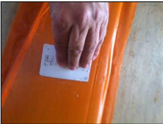
Figure 14 use old credit card to help smooth-out air bubbles
