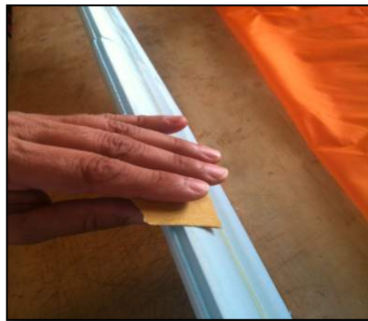
Figure 9 Sand Leading Edge foam to fit rod
