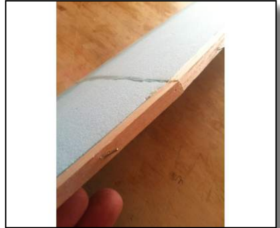
Figure 3 align leading and trailing edges
