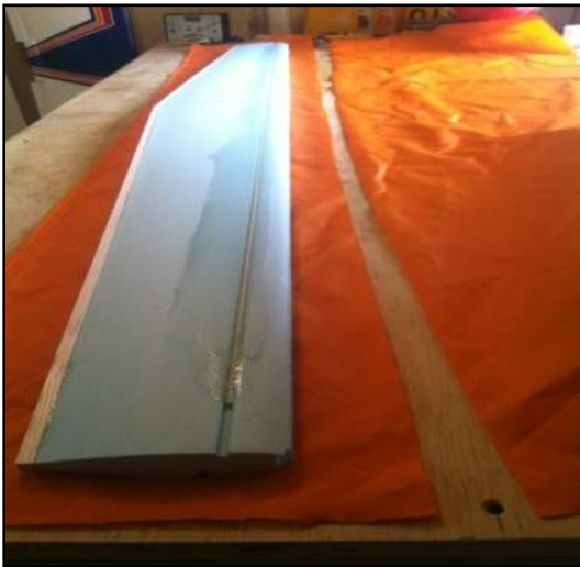
Figure 10 cut fabric to size -1"- 2" larger than foam core
