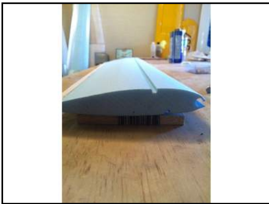
Shim wing tips and test fit wing cores
