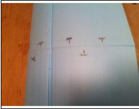
Figure 2 Glue wing halves together
