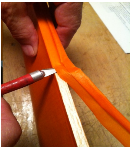
Figure 18 Trim covering around the perimeter
