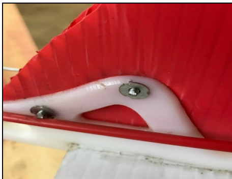
Figure 34 Vertical fin installed using 4-40 blind nuts and cap screws
