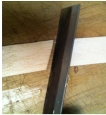
Figure 23 Trim to desired angle
