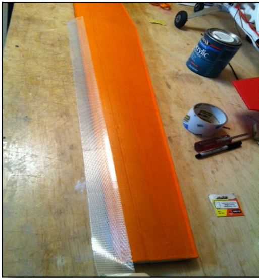
Figure 20 Tape leading edge in 2 parts
