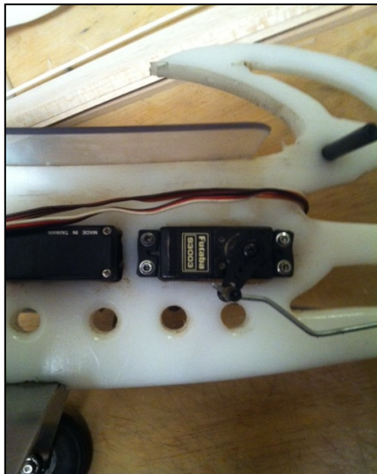
Figure 52 Throttle push rod at servo
