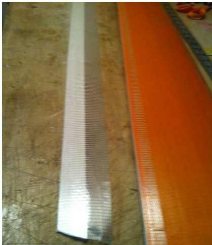
Figure 26 attach bi-directional tape - over lap first layer
