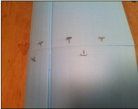
Figure 2 Glue wing halves together
