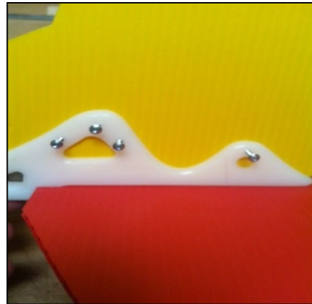
Figure 37 Vertical fin mounting screws
