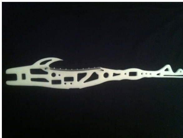
Figure 30 Fuselage with wing saddle attached
