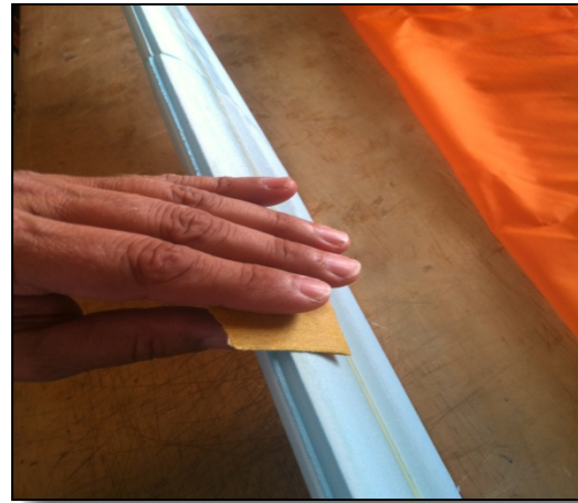
Figure 9 Sand Leading Edge foam to fit rod
