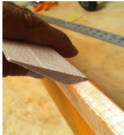
Figure 27 attach to trailing edge in deflected position
