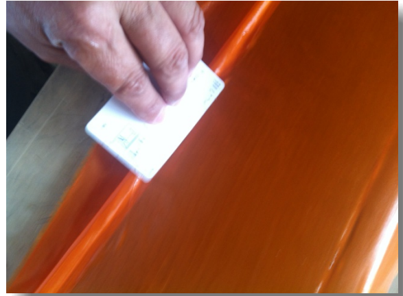
Figure 15 Move excess urethane to top of wood trailing edge
