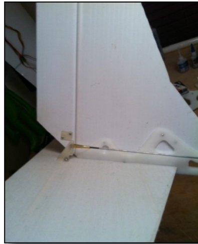
Figure 49 Elevator linkage installed
