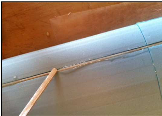
Figure 4 add plenty of epoxy to the rod and groove
