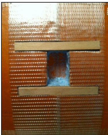
Figure 46 relive foam to accept servo mounting rails
