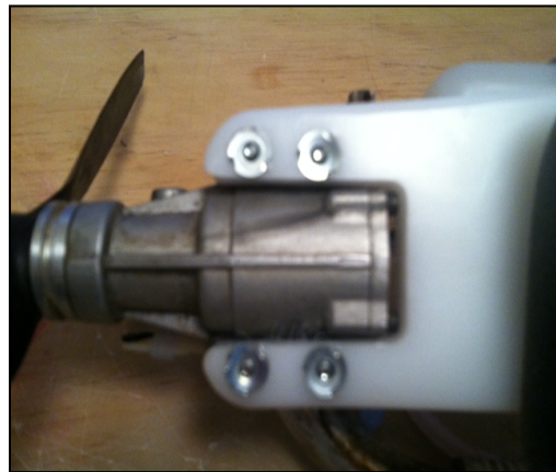
Figure 33 Mount engine with 4-40 x 3/4 inch socket head cap screws
