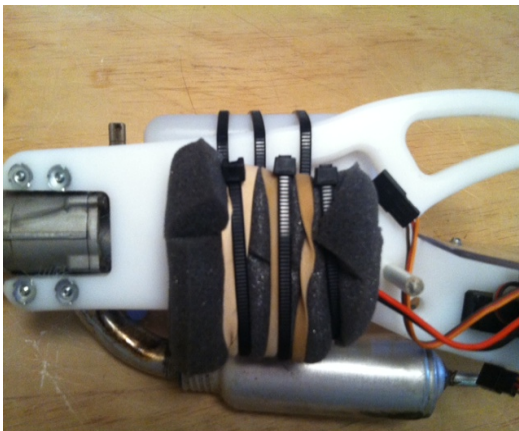
Figure 62 Battery mounted to fuselage
