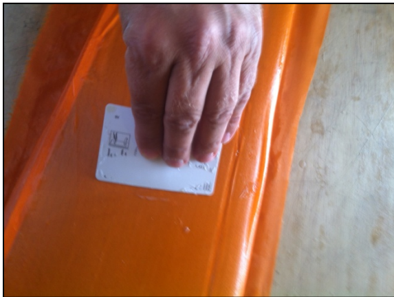
Figure 14 use old credit card to help smooth-out air bubbles
