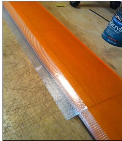
Figure 21 tape second half of leading edge
