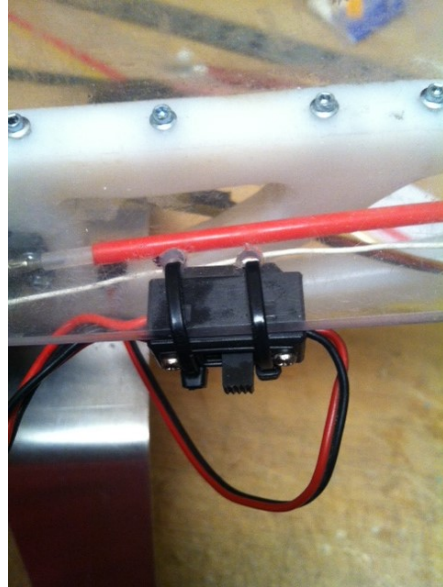
Figure 67 Switch mount on Lexan saddle, top view
