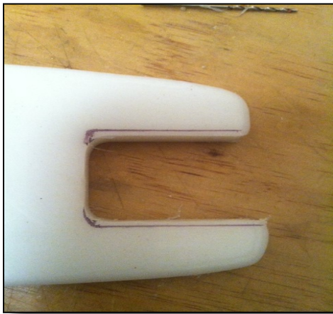
Figure 32 Mark for your engine size
