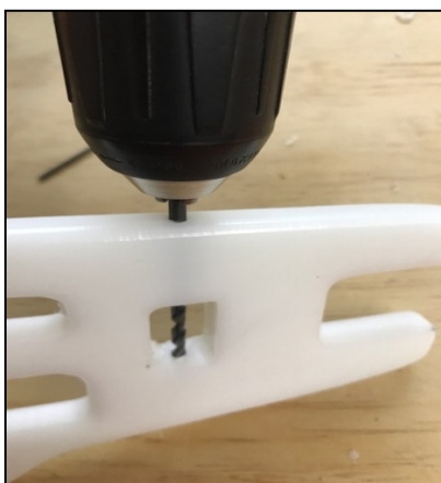
Figure 38 Drill 5/32 hole for landing gear wire
