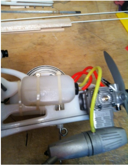
Figure 60 6 Oz. tank mounted behind engine
