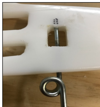
Figure 39 wire should go into upper portion of cut out
