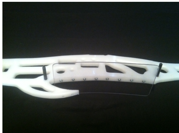
Figure 31 Wing Dowels in place
