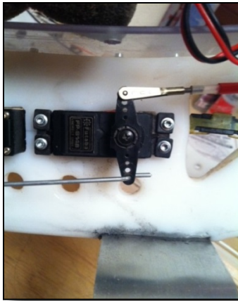
Figure 50 Rudder / steering servo mounted
