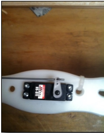
Figure 48 Elevator servo mounted with servo arm up
