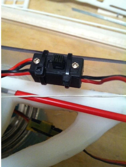
Figure 66 Switch mount on Lexan wing saddle
