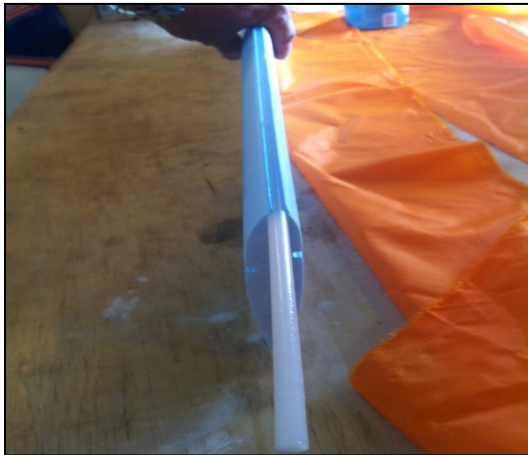
Figure 8 Insert Leading Edge plastic rod
