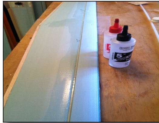
Figure 7 Properly installed fiberglass rod!
