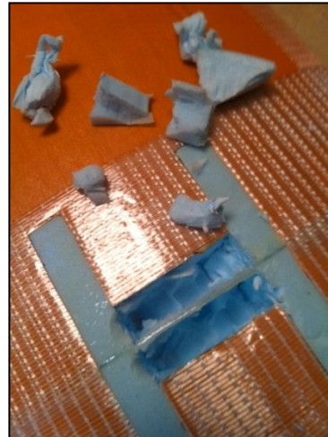
Figure 45 Remove foam from servo cavity
