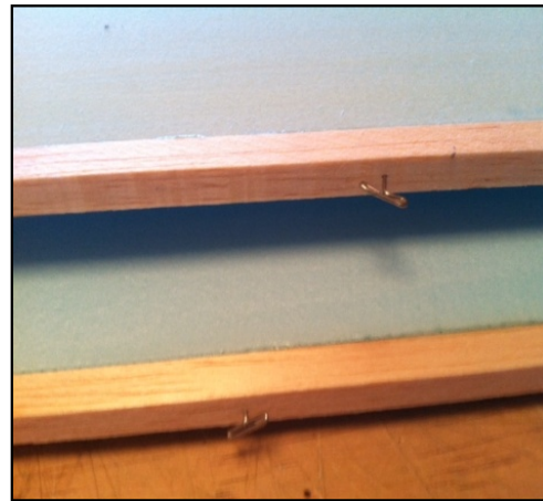
Balsa TE end caps held in place with T-pins
