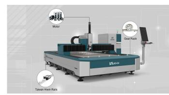
All Anvil Lx Fiber Laser Machines are available with German made Atlanta Gear Rack Systems, Japanese Yasakawa Motors and Hiwin Rails from Taiwan.
