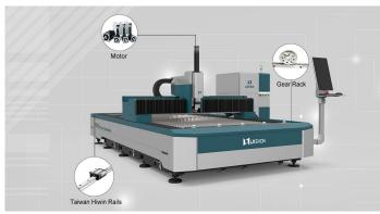
All Anvil Lx Fiber Laser Machines are available with German made Atlanta Gear Rack Systems, Japanese Yasakawa Motors and Hiwin Rails from Taiwan.
