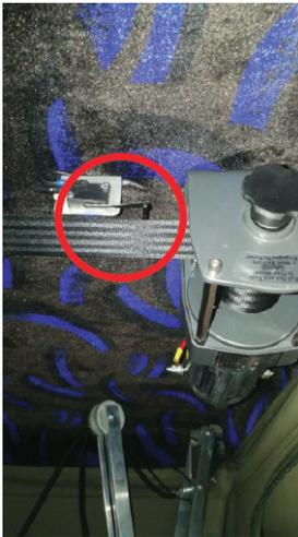
Location of Limit Switch near the winch motor
