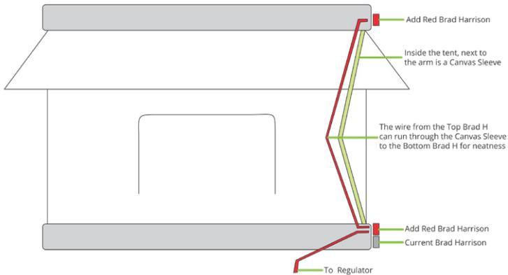
To hide wires you can run them underneath the CANVAS edging around the tent – merely lift this edging, run the wiring through and glue down neatly again (you can use the canvas sleeve in the arm to hide any additional wiring).
