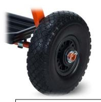
**Step 1:** Lubricate axle with oil or grease. Put the wheel on the axle. Insert washer M-50 and safeti pin.
