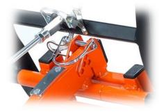
**Step 4:** Mechanical fuse is used against self closing (mandatory use)
