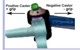
Dry conditions: Use the kart in the low position and the stub axle in the high position
