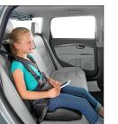
Universal postural belt system that can be used in any seat, provided there is an opening between the seat and the backrest
