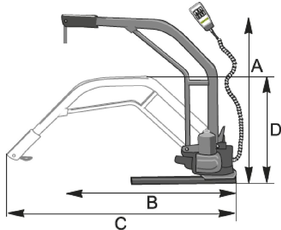
**A = 106 cm including mounting base. Height adjusted by cutting**
