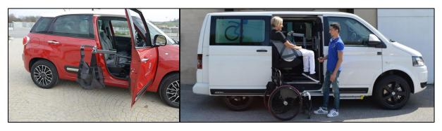
The Person lift is designed to carry someone from a wheelchair into the seat of the vehicle. By utilising a sling for the transfer the lift eliminates the strain put on the carer for transfers while safely transferring the occupant into the seat. Once you have completed the transfer the Person lift can then be stored securely in the boot of the vehicle.
