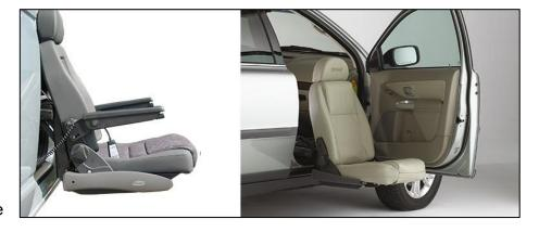
The Turny Orbit is a fully automatic swivel seat where all movements are operated by the hand held remote.
