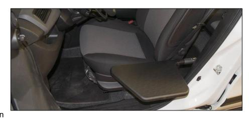
both a manual and electric version that incorporates a lifting function. As the transfer board is fixed onto the vehicle this reduces the safety risks involved with transferring and has a weight capacity of 120kg.
