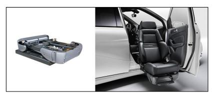
It is a fully automatic, programmable swivel seat where all movements are operated by the hand held remote. This unique programmable function means that you can set the parameters of the swivelling function to optimise the amount of room generated in the vehicle and also allows it to be installed into the drivers seating position of many vehicles.
