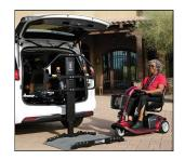
The **VSL-4400** Joey Lift allows you to ride a mobility device onto the platform from either direction, press a button and the Joey lifts and stows your device into the back of your vehicle. The Joey lift is a safe, simple solution to transport your mobility device around during your travels.
