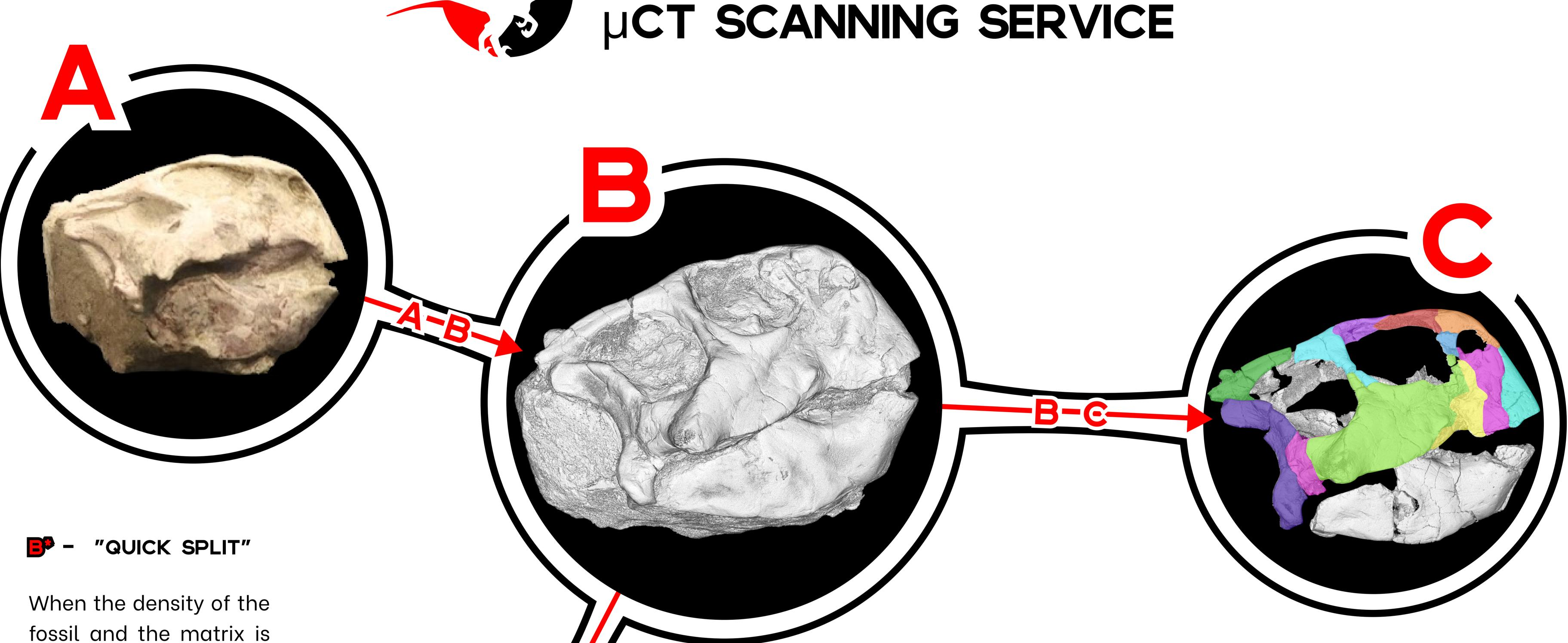
When the density of the fossil and the matrix is distinct, as found in phosphatic and some pyritic fossils, it's possible to split the two by filtering by density in the software.
