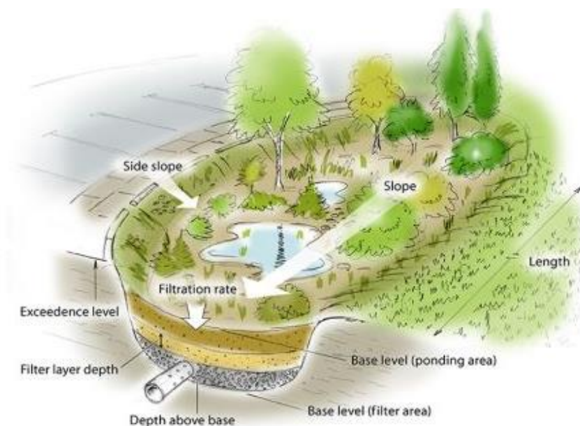
Figure-2 Designed pond (source: Suds software )
