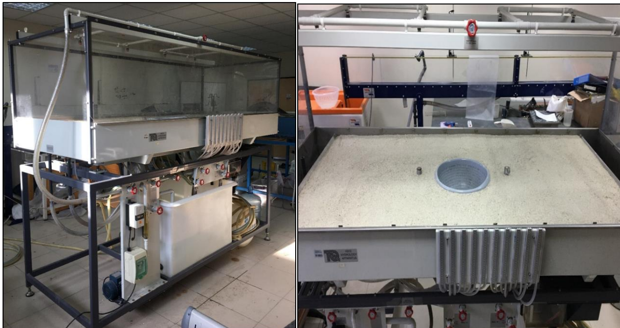
Figure1 Lake-Aquifer Interaction Experimental Setup with Hydrology Apparatus.
