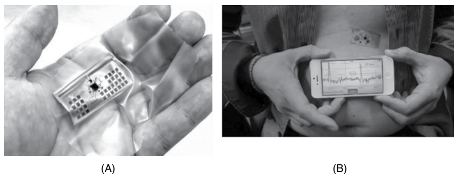
Figure 3.3 (A): The sensor fabricated on a stretchable substrate. (B): The sensor signal is delivered in real time in mobile device [11].
