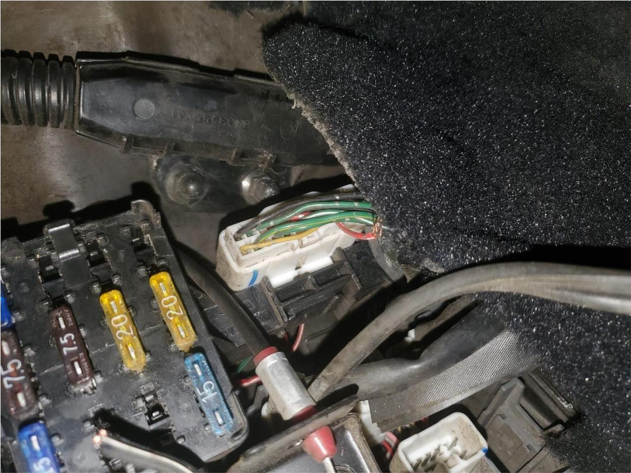
Disconnect the plugs behind the seat. It would help to remove the sound deadening on the firewall and the side cover panel. One hard to get one is the 3<sup>rd</sup> brake light you will have to chase it all the way back or cut it and reconnect later.
