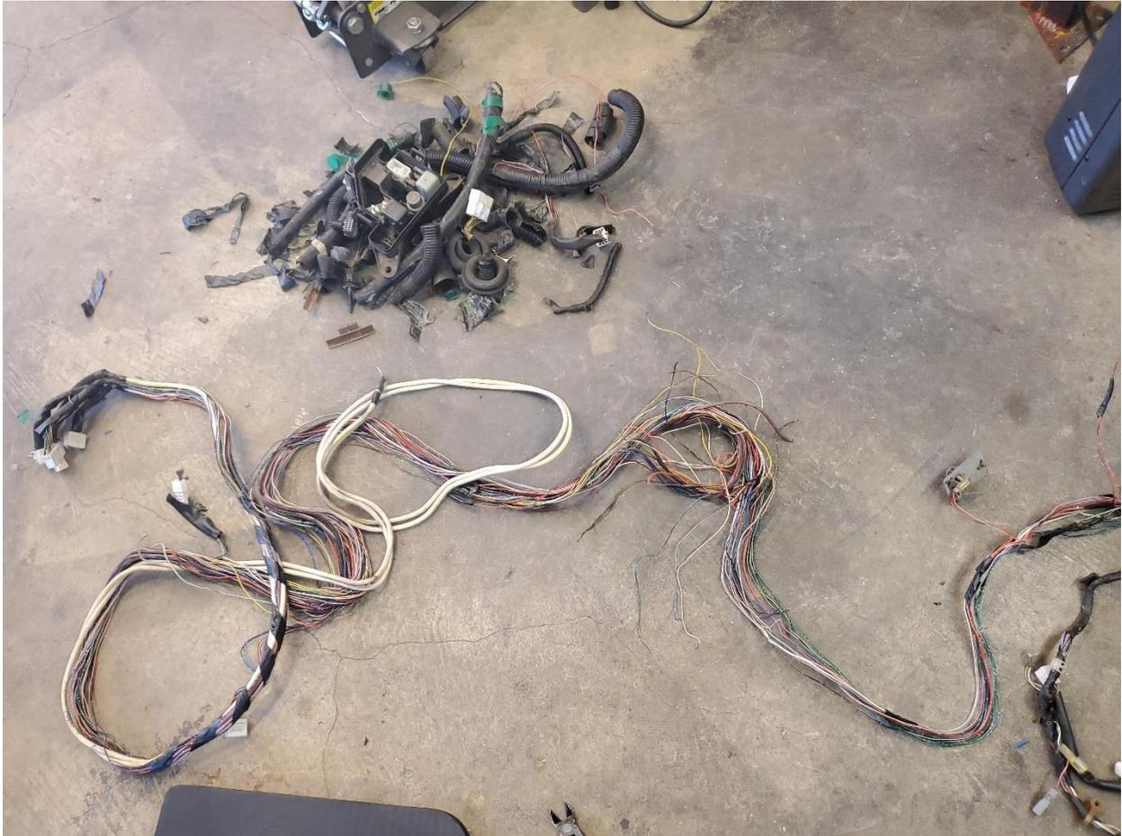
Find the color matching wires from the swap harness and pull them all aside along with the new alternator power wire. You need the wires that are going directly to the plugs at the kick panel.
