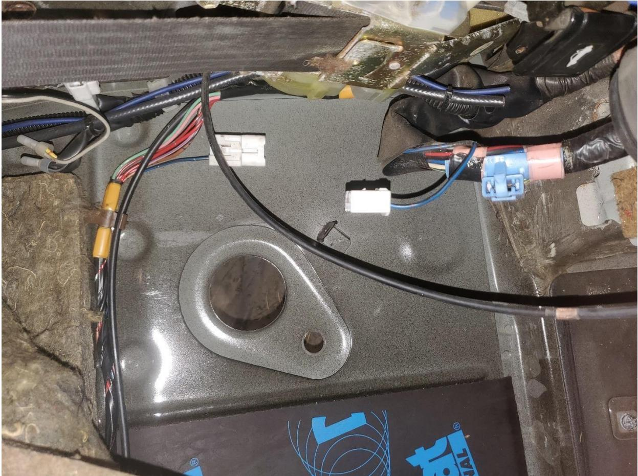
Picture above is the fuel pump power wire, thick blue.
