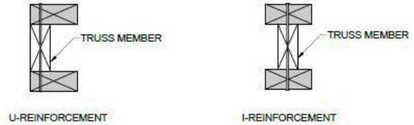
**ELEVATION VIEW OF I OR U REINFORCEMENT**
