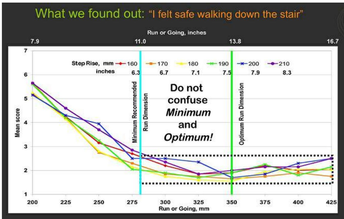
Figure 2. Results of BRE Laboratory Testing of Combinations of Step Rise
