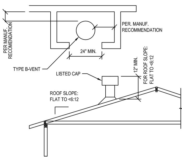
**WATER HEATER VENT AND ACCESS REQUIREMENTS**
