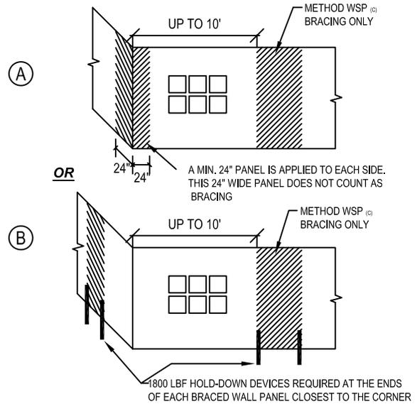
2. MIXING BRACING METHODS WITHIN A BRACED WALL LINE IS NOT PERMITTED.
