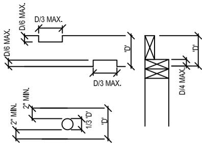
NOTCHING & BORING FLOOR JOIST
