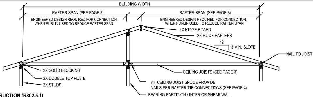
BRACED RAFTER CONSTRUCTION (R802.5.1)
