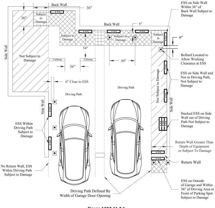
Figure 1207.11.7.1 ESS Vehicle Impact Protection
