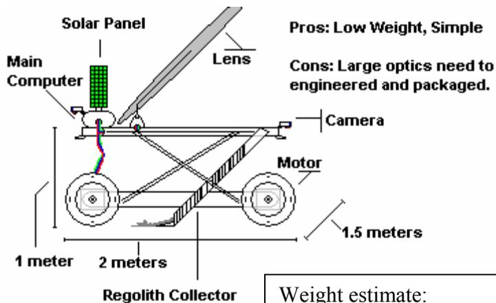
**Heliostat-type regolith fuser:**
