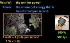
This a 60 Watt incandescent light globe and this is a 500 Watt incandescent light globe. The 500 W light globe is obviously quite a lot brighter than the 60 W light globe. But what is a Watt? What does 60 Watts, for example, mean?
