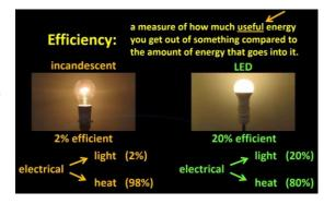
An LED light globe can generate 10 times as much light using the same amount of electricity, or the other way of thinking about it is, it can generate the same amount of light using only 1/10 of the electricity.
