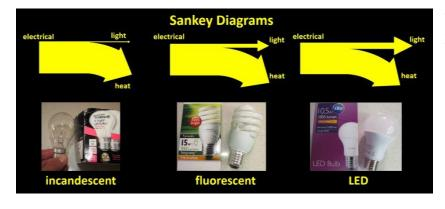
To graphically express the efficiency of a process, we often use what are called Sankey diagrams, named after Matthew Sankey, an Irish-born engineer who improved various aspects of steam engines in the late 1800s. Sankey diagrams show the energy input and energy outputs of different devices or systems in this case of three different kinds of light globes and can therefore represent graphically the energy efficiency of the device or system.
