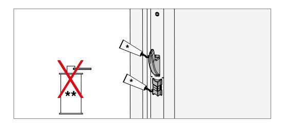
Lubricate the MF-HO locking element 1x annually!
