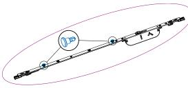
The A-TS intermediate faceplate module is delivered with two pre-inserted fixing pins!
