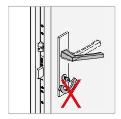
Do not simultaneously press the handle and turn the key!
