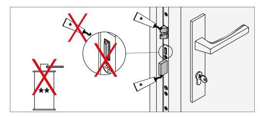
The door lock (lock case) is delivered with an intensive lubrication of high performance greases and must NOT be re-lubricated! Lubricate the latch and locking bolt 1x annually!
