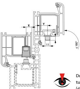
Due to the various hinge options and the resulting turning axes, the position of the cable tray (dimension X) and the cover plate (dimension Y) must be determined independently!
