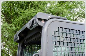
Install light guard as shown in pictures. No drilling is needed.
