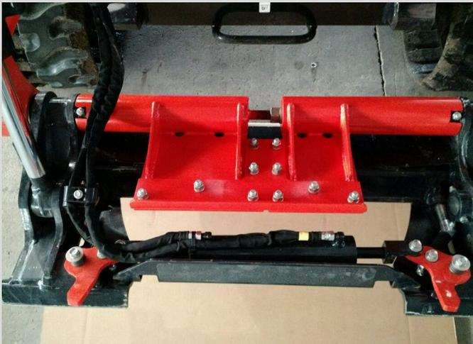
5. Install "T" shaped splice bracket as shown. Toe of top flange should face cab. \*\* Note: Stand-off plates should engage factor cross member approximately as shown in end view.
