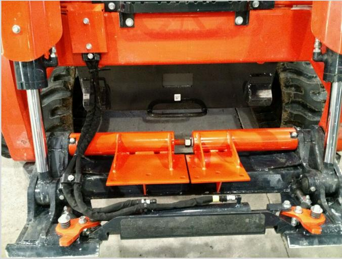
4. Hand tighten 1" hex nut. Lock washer should be on shorter half side.
