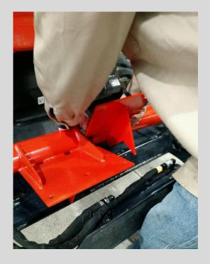
3. Repeat for smaller half. Tilt or rotate halves so that loose end of 1" stud inserts into smaller half.
