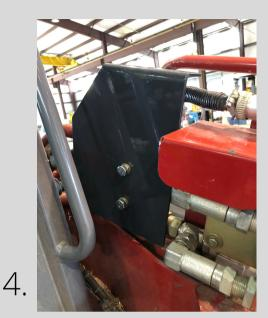
Note: Lower coupler guard mount tabs install on top of factory grab rail mounting tabs. Retain washers from factory bolts to be re-used with supplied M10x1.5mmx30mm bolts (4 each).
