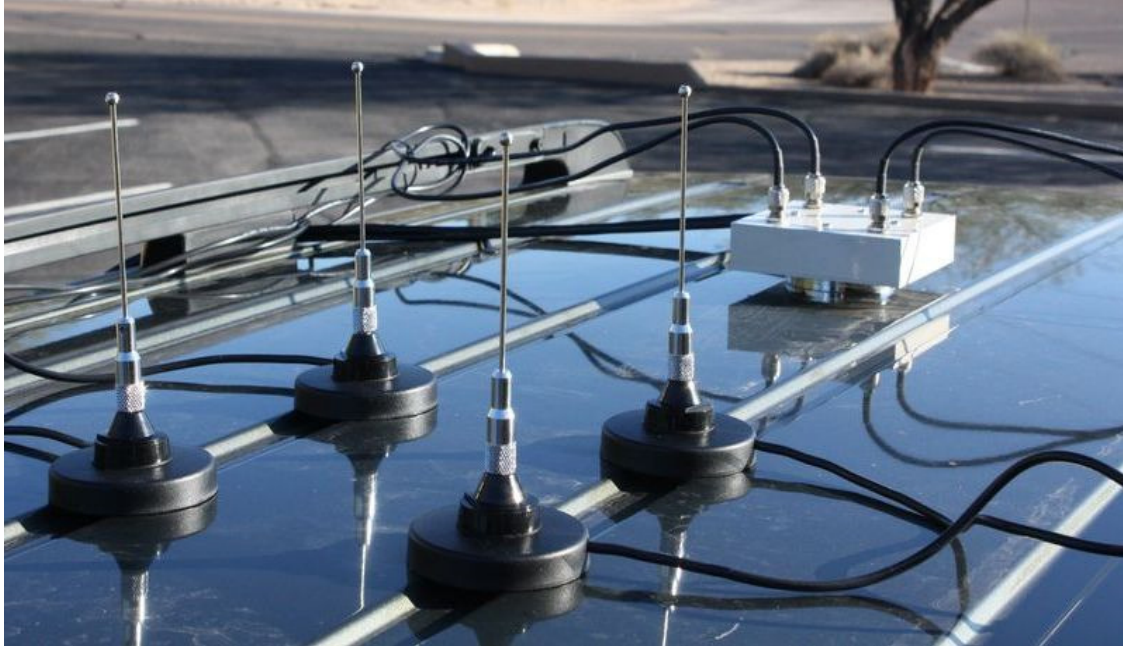
Figure 3: Mobile Antenna and Summing Unit for 250 – 500 MHz
