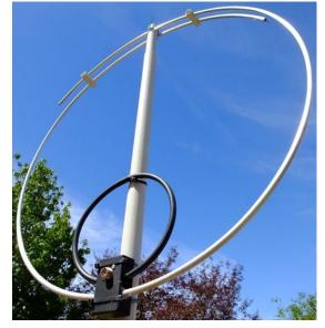
typically a loop of copper or aluminum tubing, forms a closed circuit with a variable capacitor in parallel.
