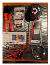
I carry a field repair kit containing basic tools including screwdrivers, pliers, wire cutters, wire crimpers. I also carry everything I need to repair a failed Anderson Power Pole connection, a multimeter (thank you harbor freight!) and a butane-fueled soldering iron (not the best, but it will do in a pinch).
