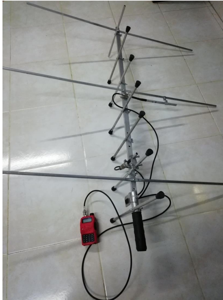
Baofeng UV-5R and homebrew 2m/70cm Yagi (courtesy XE3AA)
