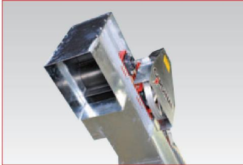
Generous discharge opening with rubber-backed end plate minimizes clogs and seed damage
