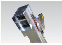
Generous discharge opening with rubber-backed end plate minimizes clogs and seed damage
