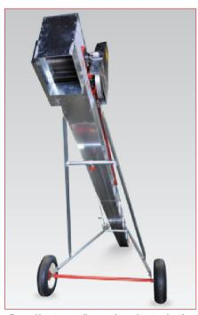
Tapered bearing spindles on axles and optional trailer rated tires allow for worry free transport.
