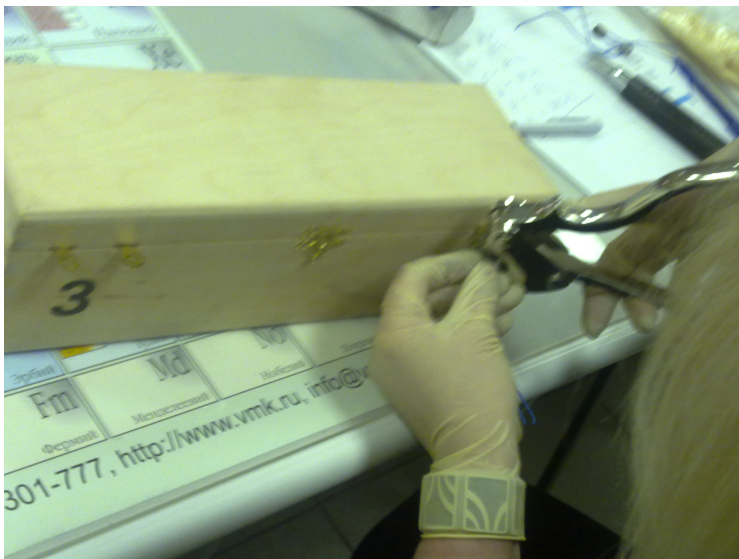
Collection of samples for analysis, labeling of the coils and box, and sealing the box.
