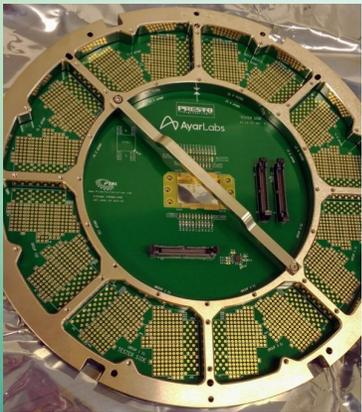
Traditional VLSI probe card -> no optical connectivity
