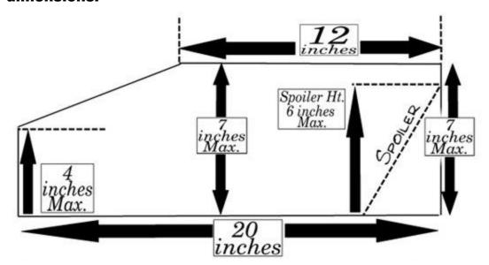
Modified spoilers may use maximum 2 side panels shaped like or similar to diagram template.
